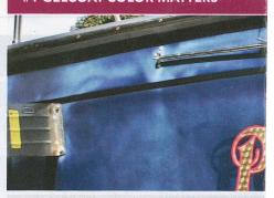
Gelcoat is a thin, pigmented, resin-rich the outside of the boat. Gelcoat has two to keep the water out of the fiberglass la to make the boat look pretty. The latter plains the reason for so many hulls in such as blue, black, red and forest green.
