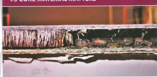
If you are buying a composite (fiberglass) boat, then you can count on two things: the hull and/or deck will have core material between fiberglass skins, and there will be elevated moisture found somewhere during the survey.
