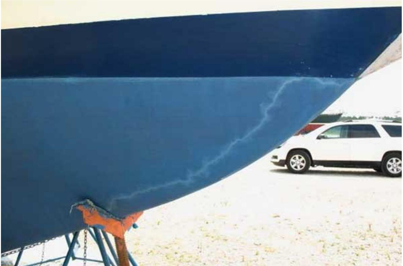
This "lightning track" shows how the electrical charge passed from the bobstay to the jackstand to reach the ground.
