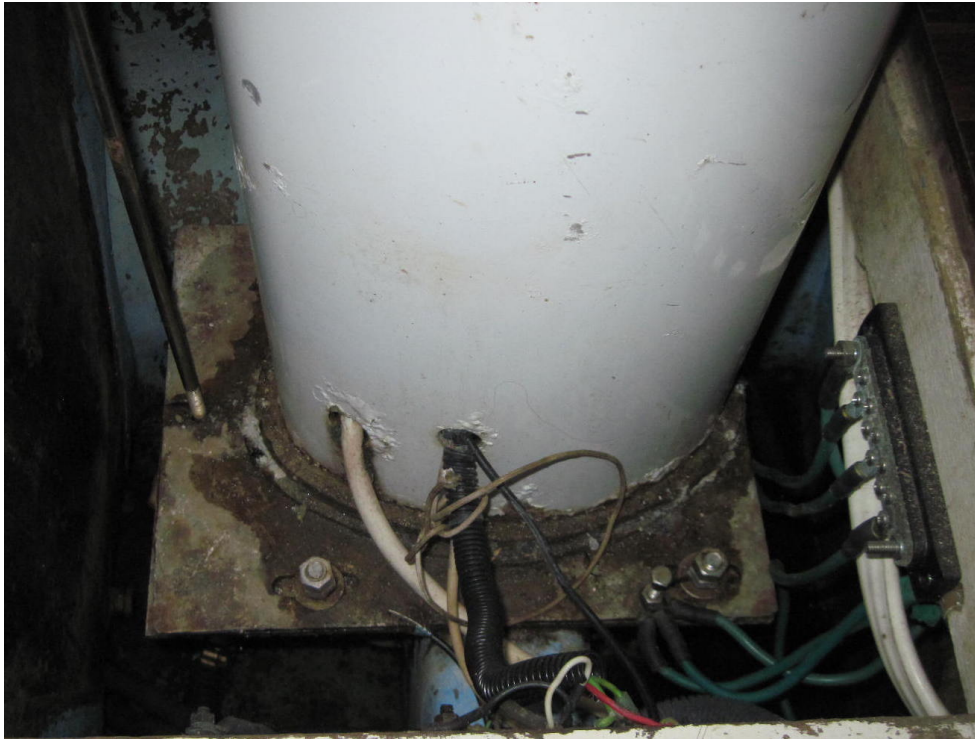
Mast Step ( Grounds / Bonding terminal block at right )
