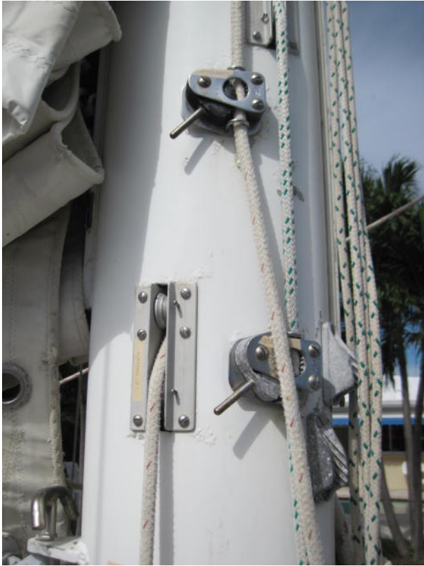
Dated mast hardware, paint bubbling.
