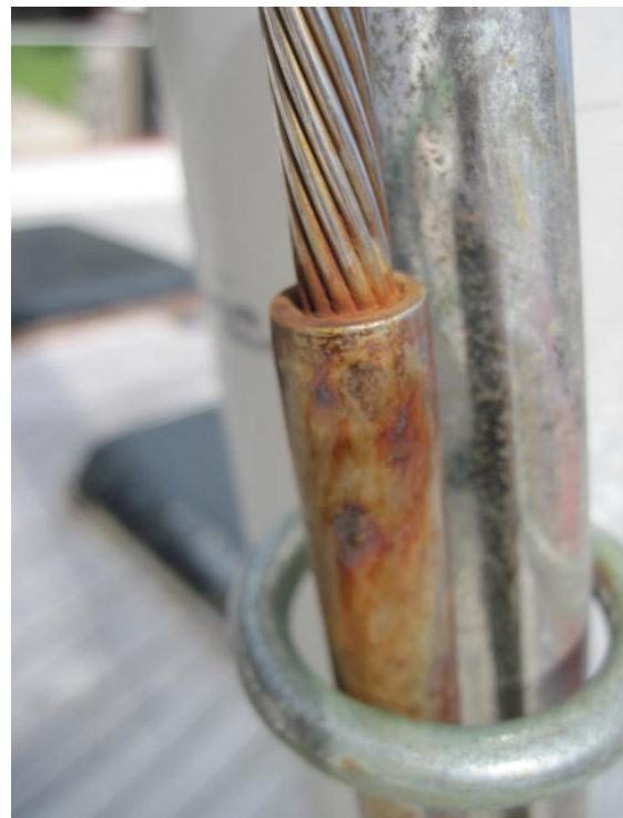
Forward lowers - heavy corrosion.
