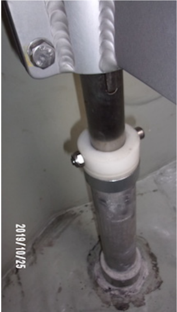
(Left) Rudder Shaft Tube & Hull Support
